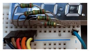
The active-low<sup>1</sup> digit-enable outputs are named en[3] through en[0] in order from left to right and the active-high segment-enable outputs are a through g (see the diagram above). For this lab only the rightmost digit is used so (en[0]) needs to be set low and the other digit enables high.
