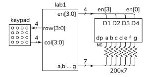
Your circuit should display one of the last three digits of *your* BCIT ID in the rightmost digit position when the keypad buttons 1, 2 and 3 are pressed. For
