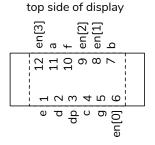
This is a common-cathode display so you must set the pin for a segment (A-G) high and the desired digit enable (DIG1 through DIG4) low to turn on that LED segment. Note that only one digit can be displayed at a time.
