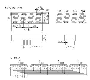
The display pinout is:
