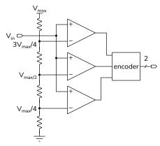
Draw a diagram showing the voltage ranges, the comparator outputs and the binary output for the 4-bit flash ADC above.
