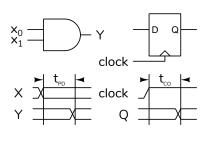
These delays are primarily caused by the time required to charge the parasitic capacitances of transistors and the metallic "interconnects" that connect them.
