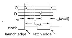
Q becomes valid  $t_{CO}$  after the first ("launching") rising clock edge. After  $t_{PD}$ , the propagation delay through the combinational logic, D will have a correct and valid logic level.
