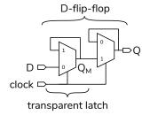
When the clock input is low, the output of the first multiplexer follows the input – the latch is "transparent". When the clock input is high, the output level is fed back to the input and held at that level.
