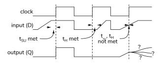
To avoid metastability we must ensure the voltage at the latch input is at valid level long enough to drive the latch output to a valid voltage level before the rising edge of the clock. The time required for this is called the "setup" time,  $t_{\rm SU}$ .
