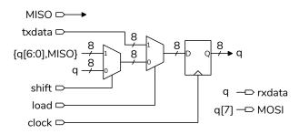
The shift register loads the eight MOSI bits to be transmitted from txdata when load is asserted. When shift is asserted a MISO bit shifts in on the right and a MOSI bit shifts out on the left. At the end of the transfer the eight received MISO bits can be read in parallel from the shift register on rxdata.
