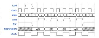
**Exercise 2:** Based on the diagram above, write a state transition table for an SPI interface controller that transfers four bits at a time. Include an idle state. In which states are SCLK and  $\overline{SS}$  asserted?
