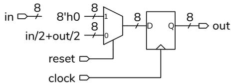
This is an example of an Infinite Impulse Response (IIR) filter.
