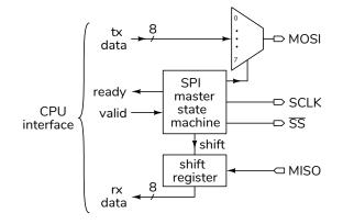
The controller is a state machine that sequences through 16 states, two for each bit (one for SCLK high and one for SCLK low).
