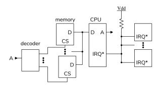
**Exercise 5:** What are the active-state current and the RC time constant for a wired-or interrupt-request line using a  $10k\Omega$  resistor pulling up a circuit with 50 pF capacitance to 3.3 V?
