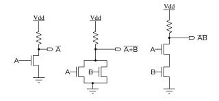
When one (for NOT), either A or B (for OR) or both A and B for (AND) inputs are high ( $>V_{th}$ ) the transistors pull the output low. The resistor (typically implemented with a transistor structure) pulls the output high otherwise.
