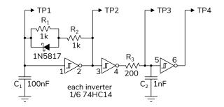
The Schmitt trigger inverter is configured as an oscillator. When the output of the inverter is high, the capacitor charges up through a 1k resistor and the Schottky diode until it crosses the upper switching threshold  $(V_{T+})$ . Then the output switches off and discharges the capacitor through both 1k resistors in series until the input crosses the lower switching threshold  $(V_{T-})$ . The different charge and discharge rates produce an asymmetrical waveform.
