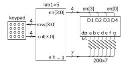
The keypad and LED pin assignments in the supplied project are the same as in the previous lab. The keypad inputs have internal pull-up resistors configured. The pin assignments are shown below:
