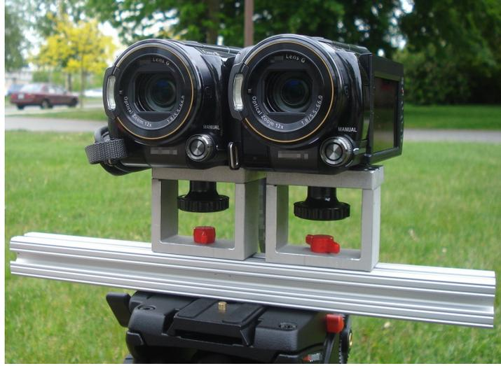
**Figure 2.1: Stereo camera setup consisting of two identical HD camcorders.**
