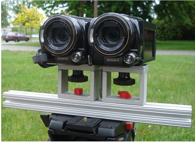
FIGURE 4 — Stereo camera setup consisting of two identical HD camcorders.
