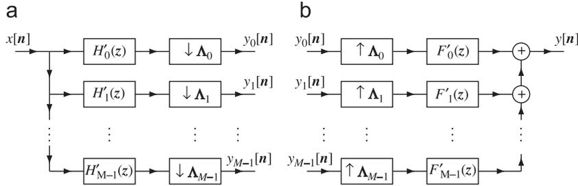
Fig. 3. The equivalent  $M$ -channel nonuniform filter bank associated with the  $L$ -level tree-structured filter bank (where  $M = 3L + 1$ ).
