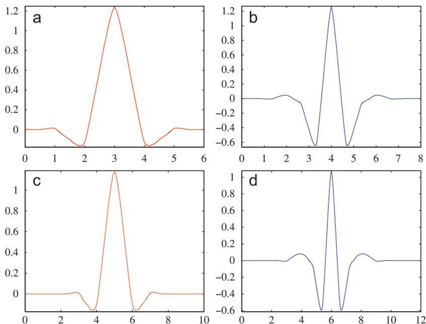
**Fig. 5.** Synthesis scaling and wavelet functions. (a) Scaling, (b) wavelet functions for the 9/7 design, (c) scaling and (d) wavelet functions for the 13/11 design.
