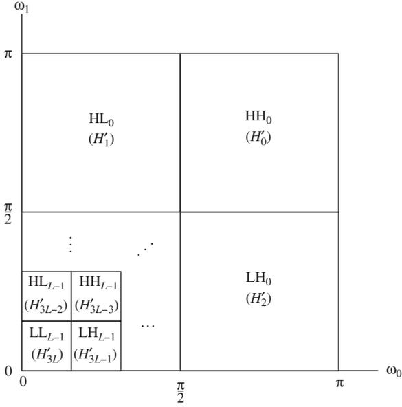
Fig. 4. Subband tiling of the first quadrant of the frequency plane.
