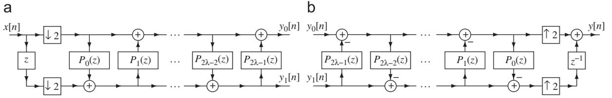
Fig. 2. The lifting realization of a 1D two-channel filter bank. (a) Analysis and (b) synthesis sides.
