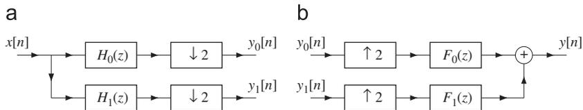
Fig. 1. The canonical form of a 1D two-channel filter bank. (a) Analysis and (b) synthesis sides.
