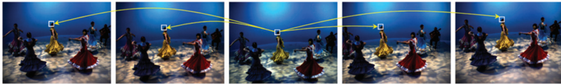
Fig. 1. Finding matching points between all views by choosing an anchor view and performing block matching between the anchor and all other.
