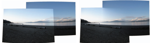
Fig. 1. Two images showing severe color mismatch aligned with no blending (left) and multi-band blending [1] (right)
