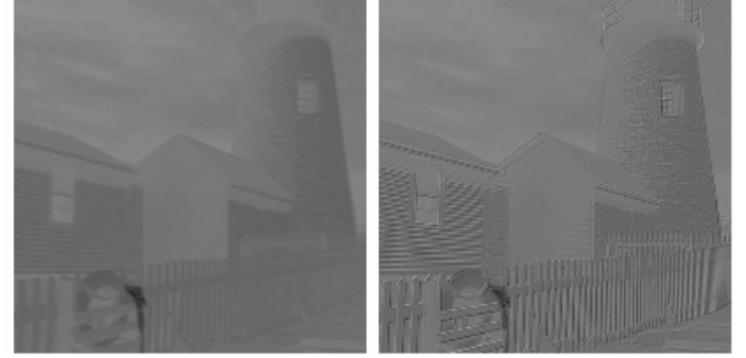
Figure 4: Cb channels of a portion of the lighthouse image. Original full colour image (left) and result of the modified YCbCr conversion used in [1]
