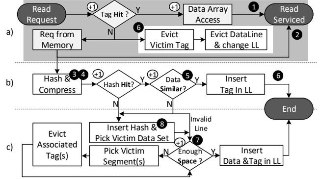
Fig. 5. Read access flowchart in 2DCC. Shaded (a) = on the critical path; unshaded (b, c) = off the critical path. LL = linked list of deduplicated tags.
