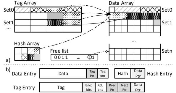
Fig. 3. (a) The three decoupled storage structures that comprise the 2DCC cache: arrows show pointers logically linking the structures. (b) Entry contents. storage or data storage, with each storage structure requiring a separate and different replacement policy.
