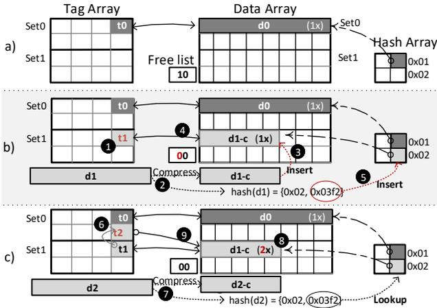
Fig. 4. Example of 2DCC operation on lines from roms\_r benchmark: (a) initial state; (b) insertion of unique but compressible block; (c) insertion of a new block whose data is identical to that of panel (b).
