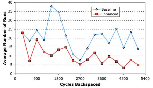
**Fig. 6:** Average processor runs per correlation sample interval for the 8051 running `sqrt`. Enhanced is the BackSpace algorithm using the algorithm proposed in Section 4 of this paper.
