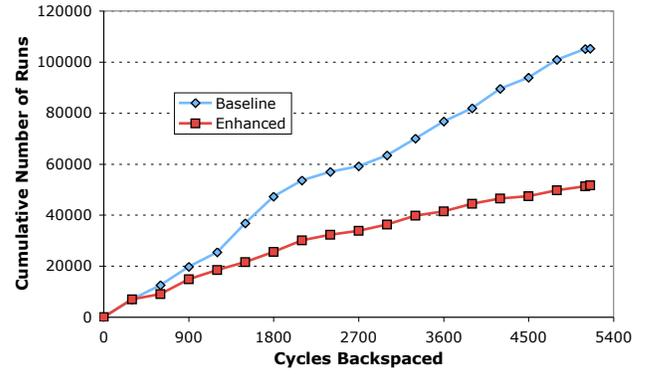
**Fig. 3:** Cumulative processor runs for the 8051 running `sqrt`. Baseline is the original BackSpace algorithm. Enhanced is the BackSpace algorithm using the algorithm proposed in Section 4 of this paper.
