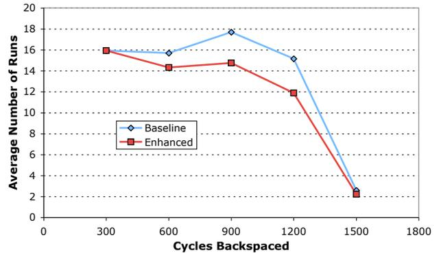
**Fig. 8:** Average processor runs per correlation sample interval for the 8051 running `fib`.
