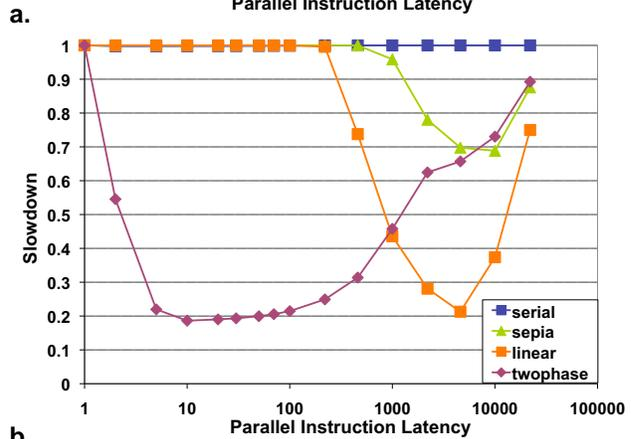
**Figure 6. Slowdown of infinite communication cost (NoSwitch) compared to zero communication cost. Real benchmarks (a), Microbenchmarks (b).**
