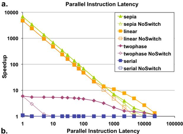
**Figure 5. Speedup of Heterogeneous System: (a) Real benchmarks, (b) Microbenchmarks. Ideal communication (solid), communication forbidden (dashed, NoSwitch).**
