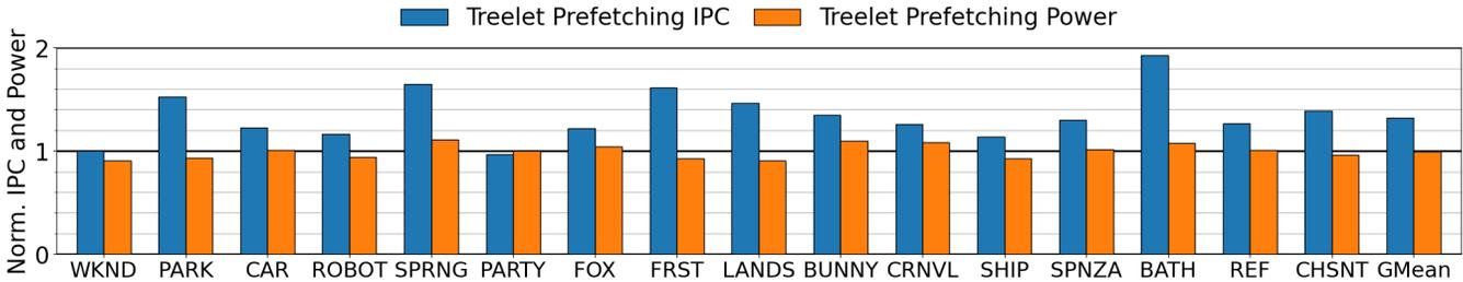
**Figure 7: Overall speedup and power consumption of treetlet prefetching with the ALWAYS heuristic, PMR scheduler and a 512B max. treetlet size.**
