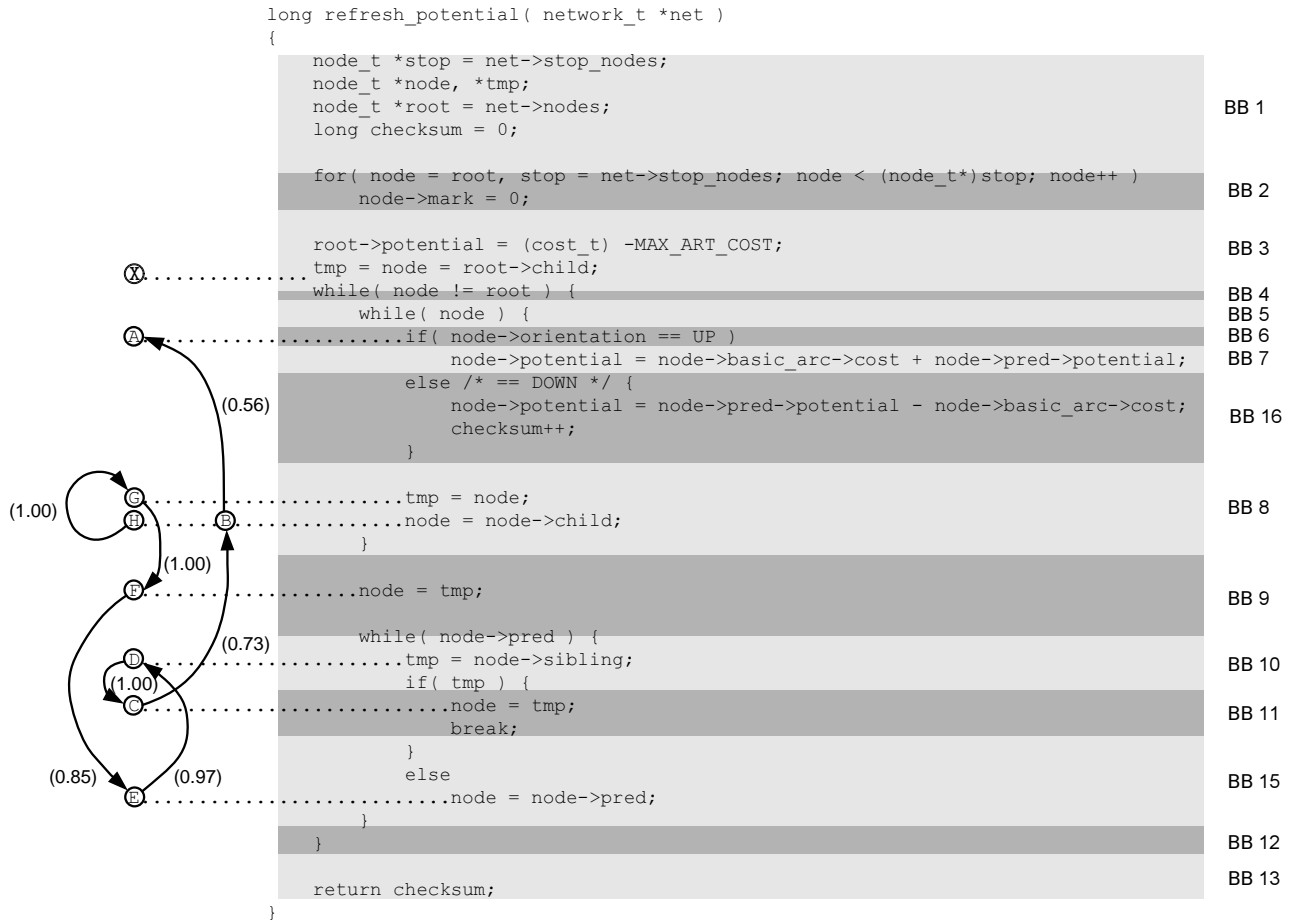
Figure 5.5: Code excerpt from Figure 5.1 with basic blocks in the gcc-2.6.3 optimized, SimpleScalar program binary.
