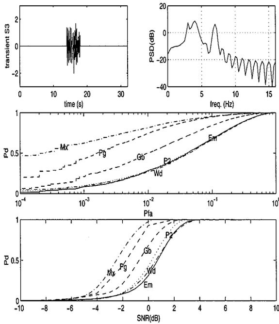
Fig. 3. Example of transient signal  $S_3$ : the sum of three exponentially decaying sinusoids with differing onsets.
