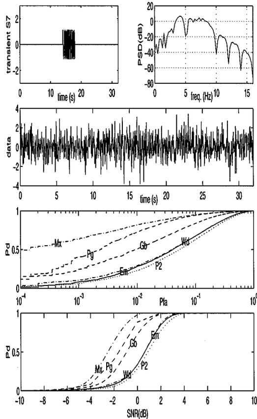
Fig. 7. Example of transient signal  $S_7$ : the tone with a stepped frequency modulation. The “data” trace in this plot exemplifies for all transient types the signal as it would look, with noise added, at the SNR used for the ROC simulation.
