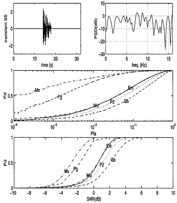
Fig. 5. Example of transient signal  $S_5$ : the exponentially enveloped white burst.
