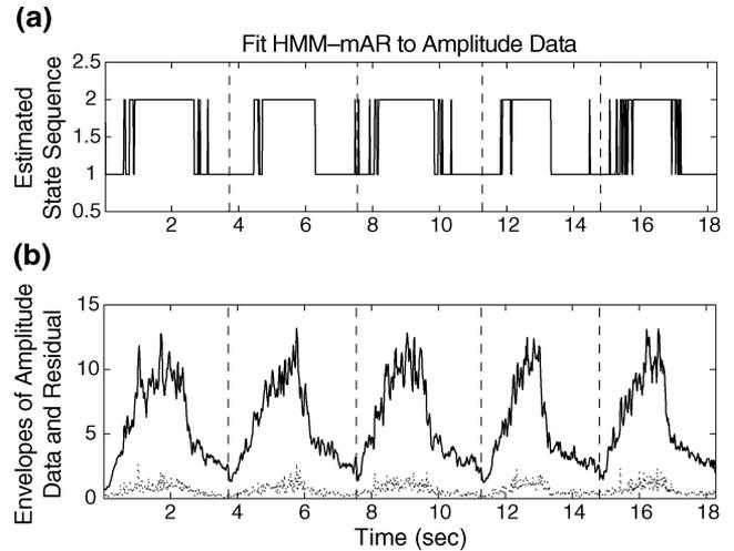
Fig. 6. Fitting a fourth-order HMM-mAR model to the amplitude component of sEMG data from the same stroke subject as in Fig. 5. The top panel (a) shows the estimated state sequence which is more stable than the case of raw data as shown in Fig. 5. Moreover, the estimation performance has greatly improved as indicated by the significant reduction in the magnitude of the residual (dotted line in the bottom panel).
