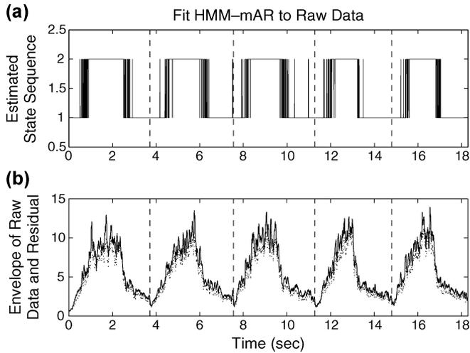
Fig. 5. Fitting a fourth-order HMM-mAR model to raw sEMG data obtained from a stroke subject over five consecutive reaching trials. The top panel (a) shows the estimated state sequence of a 2-state hidden Markov chain. The bottom panel (b) shows the envelopes of the raw sEMG data (solid line) and the residual of the fitted HMM-mAR model (dotted line).
