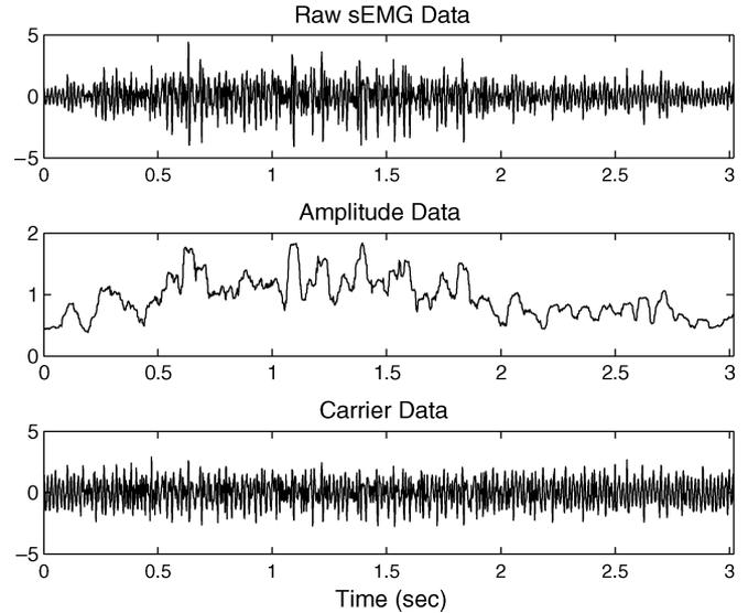
Fig. 2. Three forms of sEMG signal: raw sEMG data, amplitude data, and carrier data.
