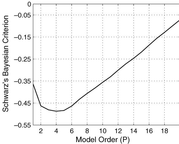
Fig. 4. Model order selection using the Schwarz's Bayesian Criterion. The optimal order is the one which gives the lowest SBC, and it is around  $P = 4$  in this case.
