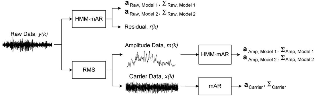
Fig. 3. Flowchart summarizing processing steps performed on various form of sEMG data.
