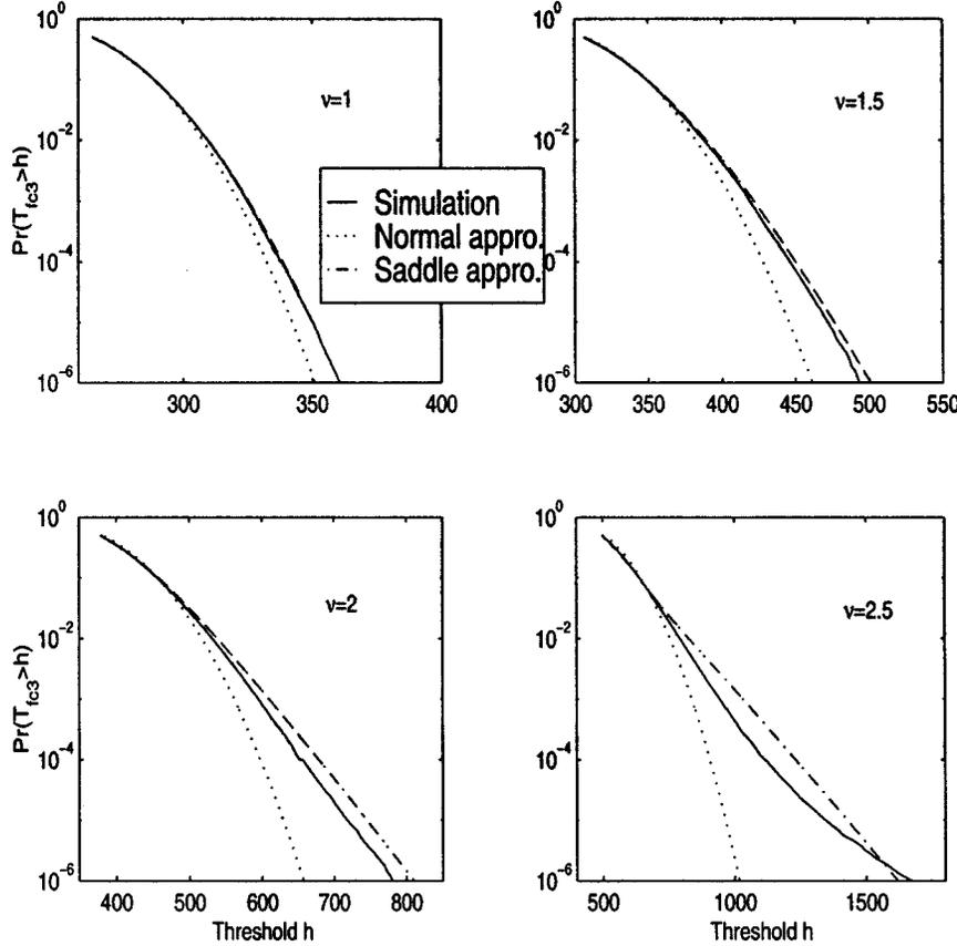
Fig. 6. Exceedance probability of  $T_{fc3}$  with normal and saddlepoint approximation as a function of threshold  $h$ . Here,  $N = 256$ , and  $L = 10$ . The right-truncated distribution is used in the implementation of saddlepoint approximation, and  $T = 10^\nu$ . The approximation results are compared with the simulation results represented by the solid line.
