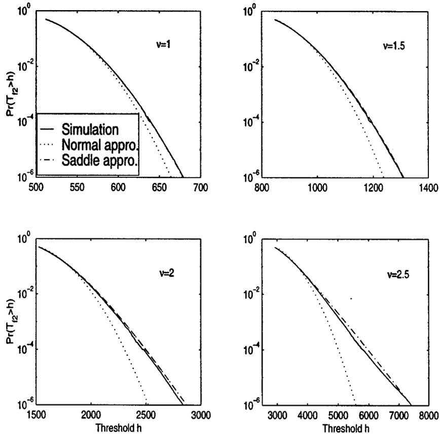
Fig. 5. Exceedance probability of  $T_{f2}$  with normal and saddlepoint approximations as a function of threshold  $h$ . The right-truncated distribution is used in the implementation of saddlepoint approximation. Here,  $N = 256$ , and  $T = 20^\nu$ . The approximation results are compared with the simulation results represented by the solid line.
