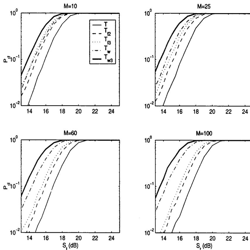
Fig. 8. Detection performances of new power-law statistics in the frequency and the wavelet domains in the prenormalized case. The exponent in each case is  $\nu = 2.5$ , and the transient duration is  $M_t = 20$  samples; different panels refer to the number of frequency bins occupied by the signal.
