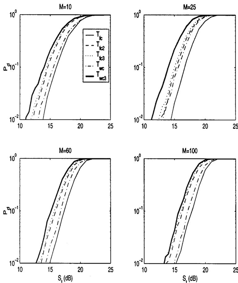
Fig. 11. Detection performance of power-law detectors in the frequency and the wavelet domains for transient detection in colored noise. Here, the time-domain transient length is  $M_t = 50$ , and the exponent used in all cases is  $\nu = 1.5$ .
