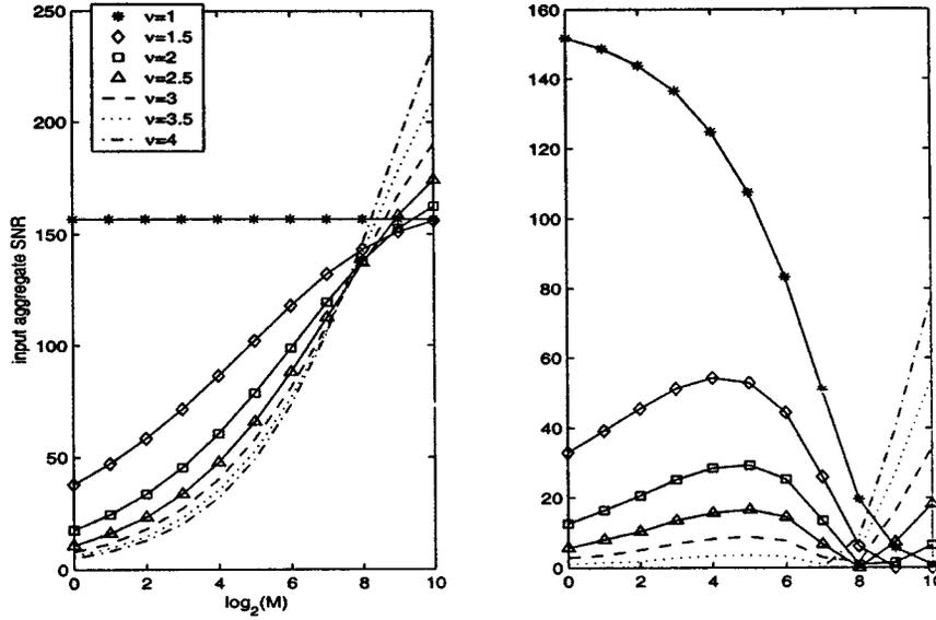
Fig. 2. SNR analysis for Nuttall's power-law statistics, with settings output  $SNR = 24$ ,  $N = 1024$ . (Left) Required input aggregate SNR for power-law detectors with different  $\nu$ . (Right) Input SNR-loss for different  $\nu$ .
