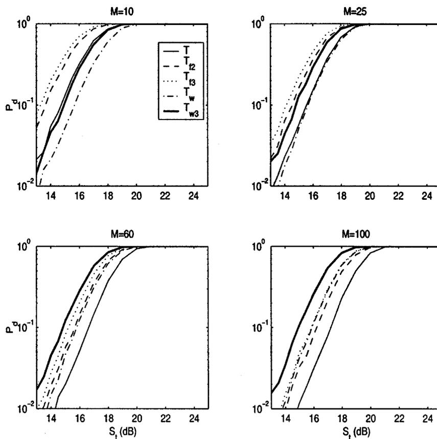
Fig. 9. Detection performances of new power-law statistics in the frequency and the wavelet domains in the prenormalized case. The exponent in each case is  $\nu = 2.5$ , and the transient duration is  $M_t = 50$  samples; different panels refer to the number of frequency bins occupied by the signal.
