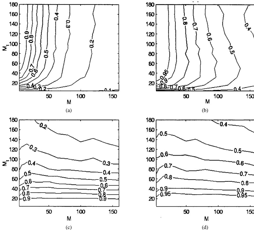
Fig. 10. Probability of detection contours for (a)  $T_f$ , (b)  $T_{f3}$ , (c)  $T_w$ , and (d)  $T_{w3}$ . These are plotted versus transient length  $M_t$  and number of signal-occupant frequency bins  $M$ .
