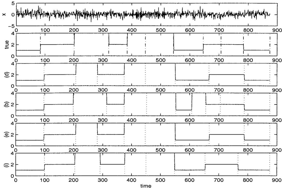
Fig. 4. Results of our scheme on the segmentation and classification of multiple structures, where  $K = 10$ ,  $L_{\min} = 32$ ,  $L_{\max} = 120$ . Top: time-series. Next: true model, out of the menu 1, 2 and 4 (see (29)). (d): Results for the time-series  $\{x_1, x_2, \dots, x_N\}$  via the DP method. (b): Using the simplified GLR method of Section III-A. (e): Using the refined scheme of Section III-B. (i): Using the iterative approach of Appendix A.
