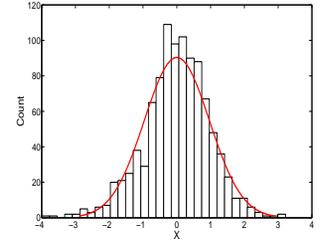
Fig. 7. A typical histogram of the time-distribution of the “carrier” signal  $x(t)$  of a muscle. The distribution of  $x(t)$  in the time domain is almost Gaussian.
