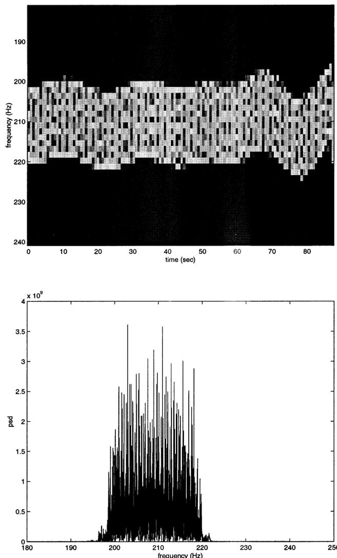
Fig. 13. Simulated signal with 10 coherently-modulated tones in 200–220 Hz range. Aggregate SNR is here 70 dB, sampling frequency is 6 kHz, and frequency modulation is of high amplitude. Above: time-frequency plot. Below: magnitude-squared FFT of length  $2^{19}$ . This is not the situation of interest in this paper, and the figure is for illustration only.
