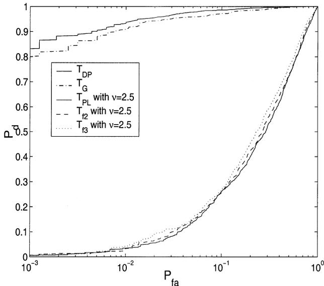
Fig. 6. ROCs of detectors for signal with frequency band [0.3, 0.31]. Aggregate SNR = 400.  $T_{DP}$  represents GLRT based on DP,  $T_G$  for our wavelet-based GLR scheme,  $T_{PL}$  for basic power-law detectors,  $T_{I2}$  and  $T_{I3}$  for combining 2 and 3 contiguous FFT bins, respectively.
