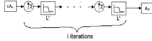
Fig. 4. Reconstructing  $i$ th level approximation  $A_i$  from coefficient vector  $cA_i$ .  $L'$  is reconstruction low-pass filter associated with decomposition filters in Fig. 3.
