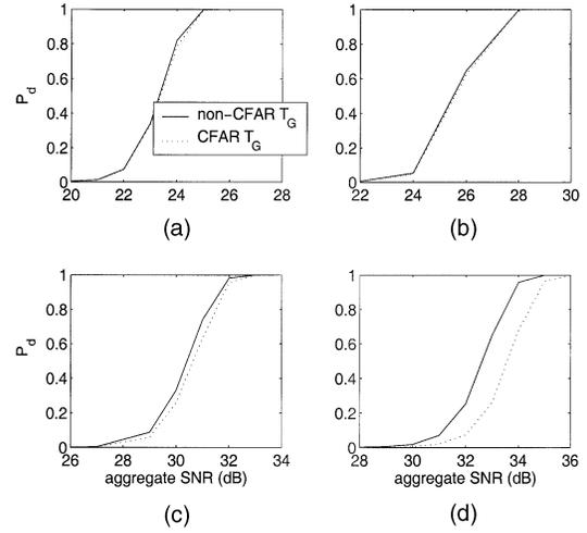
Fig. 10. Detection performance of our CFAR detector for prewhitened signals with different frequency bands. Here  $T_G$  represents our wavelet-based GLR scheme. (a) Frequency band is  $[0.2, 0.203]$ . (b) Frequency band is  $[0.3, 0.31]$ . (c) Frequency band is  $[0.3, 0.4]$ . (d) Frequency band is  $[0.2, 0.5]$ .
