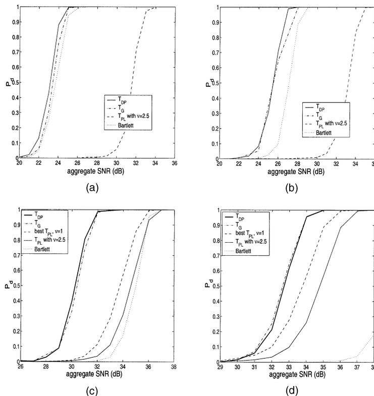
Fig. 7. Detection performance of basic detector  $T_G$  (from Section III) for signals with different frequency bands. (a) Frequency band is [0.2, 0.203]. (b) Frequency band is [0.3, 0.31]. (c) Frequency band is [0.3, 0.4]. (d) Frequency band is [0.2, 0.5].
