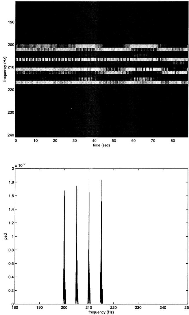
Fig. 12. Simulated signal with 4 coherently modulated tones in 200–220 Hz range. Aggregate SNR is here 70 dB, sampling frequency is 6 kHz, and frequency modulation is of low amplitude. Above: time-frequency plot. Below: magnitude-squared FFT of length  $2^{19}$ . This is not the situation of interest in this paper, and the figure is for illustration only.
