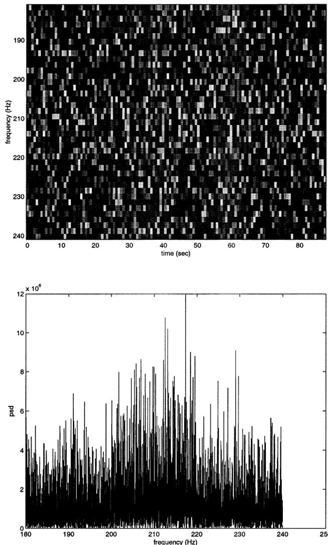
Fig. 14. Simulated signal with 100 coherently-modulated tones in 200–220 Hz range. Aggregate SNR is here 30 dB, sampling frequency is 6 kHz, and frequency modulation is of low amplitude. Above: time-frequency plot. Below: magnitude-squared FFT of length  $2^{19}$ . This is the situation of interest in this paper.
