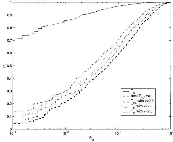
Fig. 8. Detection performance of detector  $T_G$  (from Section IVA) for signal with multiple frequency bands. Aggregate  $SNR = 1200$ , and number of bands  $M$  set to 3. Power-law detector with  $\nu = 1$  provides best performance.
