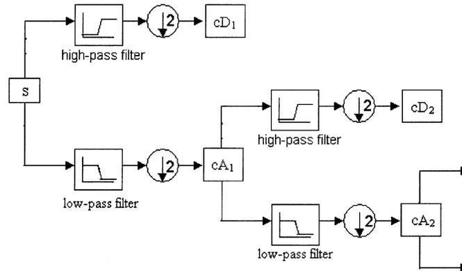
Fig. 3. Multiple-level wavelet decomposition.  $S$  means the signal,  $cA_i$  indicates approximation coefficients at  $i$ th level,  $cD_i$  indicates corresponding detail coefficients.
