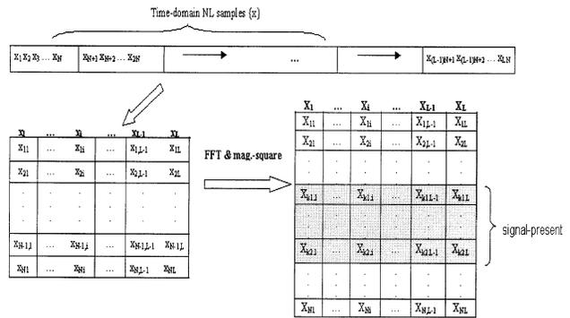
Fig. 1. Illustration of data preprocessing. Long data record is reshaped to a matrix, and DFT is applied columnwise.
