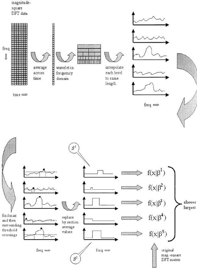
Fig. 2. Illustration of entire estimation/GLRT processing flow. Data is first arranged in magnitude-square DFT matrix according to Fig. 1, in the upper left. Wavelet decomposition is suggested in Fig. 3. Interpolation phase is performed according to Fig. 4.
