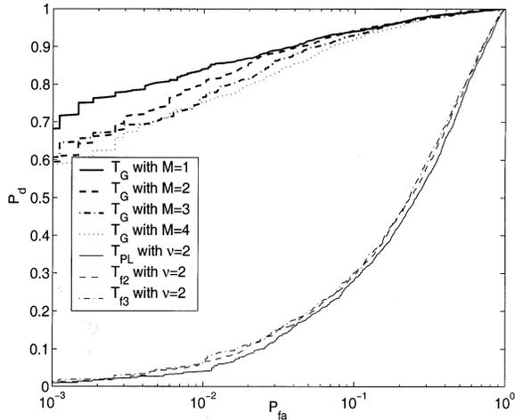
Fig. 9. Detection performance of detector  $T_G$  for signal when an incorrect assumption about number of bands  $M$  is made. Here the true band is  $[0.3, 0.32]$ , and aggregate  $SNR = 500$ . Power-law detector with  $\nu = 2$  provides the best performance.
