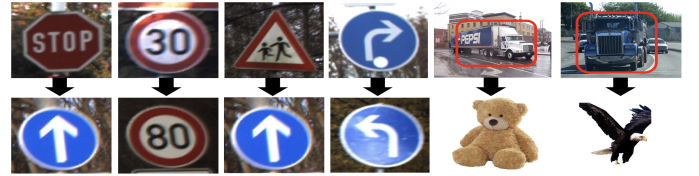
Figure 5: Single-bit flip outcome on the classifier models. Images at the first row are the input images, those at the second row are the faulty outputs.
