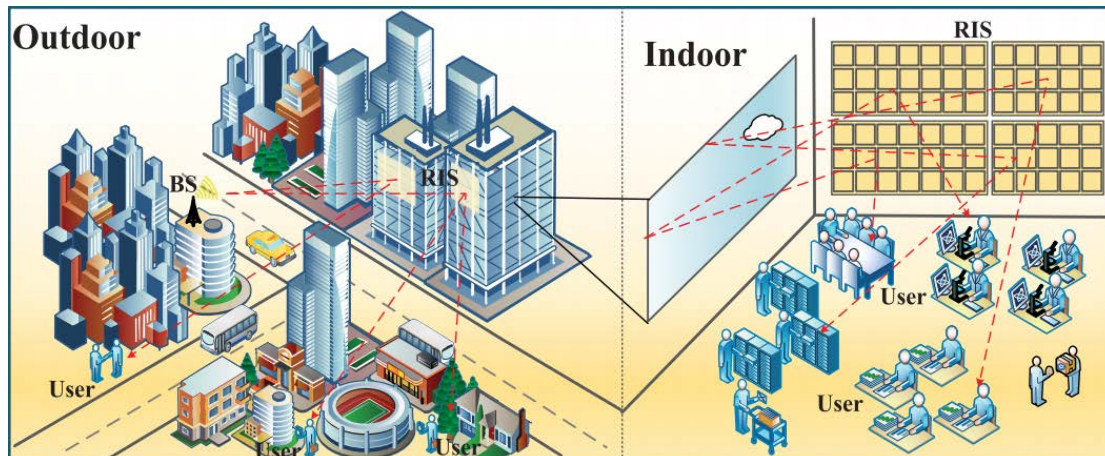
Figure 3. Outdoor and indoor applications of IRS-aided wireless communication [19]
