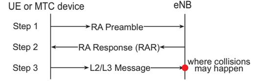
Fig. 2. The first three steps of random access in LTE networks. Multiple UEs or MTC devices may receive the same RAR if they send the same preamble in the same random access slot, so their L2/L3 messages may be transmitted on the same wireless channel and packet collisions may occur at the eNB.
