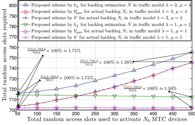
Fig. 9. Total random access slots required to serve  $N_0$  MTC devices versus the number of random access slots used to activate  $N_0$  MTC devices. ( $N_0 = 30000$ ,  $R = 1$  km,  $m = 64$ )
