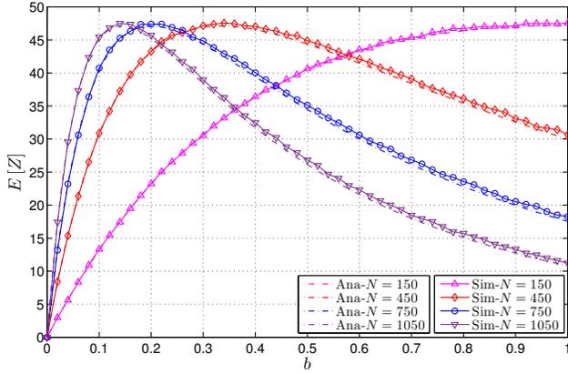
Fig. 4. Analytical and simulation results of the expected number of MTC devices served  $\mathbb{E}[Z]$  in a random access slot with different ACB parameters.
