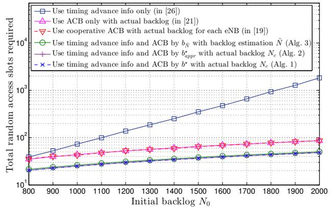
Fig. 7. Total random access slots required versus initial backlog  $N_0$ . ( $R = 1$  km,  $m = 64$ )
