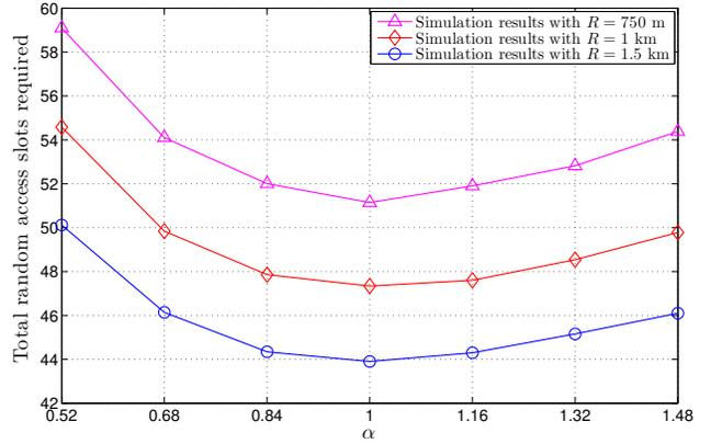
Fig. 5. Total random access slots required versus  $\alpha$  and different deployment range  $R$ . The optimal ACB parameter  $b^*$  (i.e., when  $\alpha = 1$ ) requires the minimum number of random access slots to serve all MTC devices. ( $N_0 = 2000$ )
