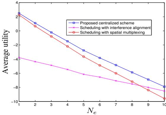
Fig. 4. Two-cell model: the average utility versus the number of cell-edge users  $N_e$  for  $P_T = 20$  dBm and  $d = 1$  km.
