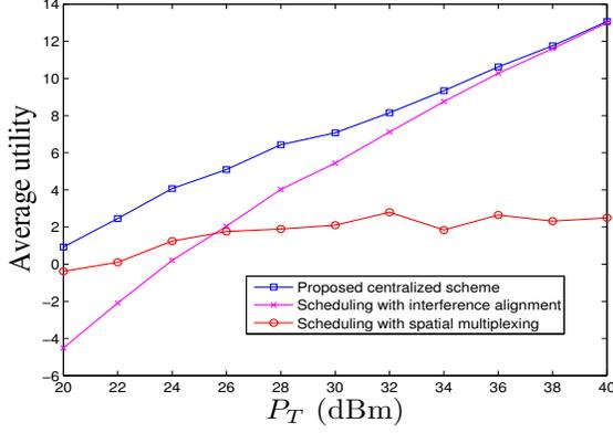
Fig. 8. Three-cell model: the average utility versus transmission power  $P_T$  for perfect CSI.
