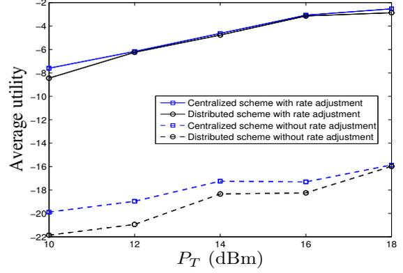
Fig. 9. Three-cell model: the average utility versus transmission power  $P_T$  for imperfect CSI for  $\xi_0 = 0.05$ .
