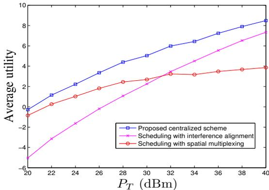
Fig. 2. Two-cell model: the average utility versus transmission power  $P_T$  with  $d = 1$  km and  $N_e = 3$ .
