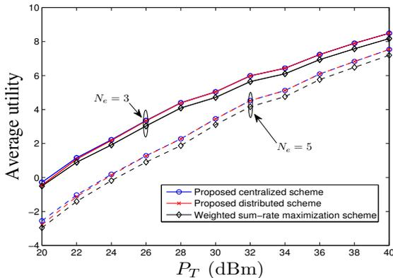
Fig. 5. Two-cell model: the average utility versus transmission power  $P_T$  for  $d = 1$  km and  $N_e = 3, 5$ .
