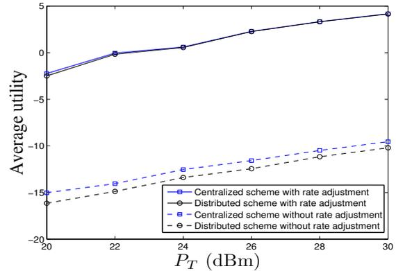
Fig. 6. Two-cell model: the average utility versus transmission power  $P_T$  for  $\xi_0 = 0.05$ .
