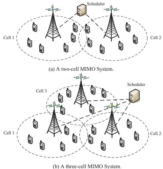
Fig. 1. Multi-cell MIMO systems. (a) Two-cell case; (b) Three-cell case. Each cell  $i \in \mathcal{I}$  has  $K_i$  users.
