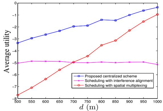
Fig. 3. Two-cell model: the average utility versus the distance  $d$  for  $P_T = 20$  dBm and  $N_e = 3$ .
