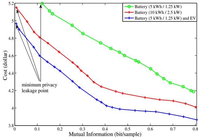
Fig. 6. Cost versus mutual information for different batteries (maximum capacity  $C_B$  / maximum charging rate  $q_B^{\max}$ ) with and without the use of an EV for load hiding.
