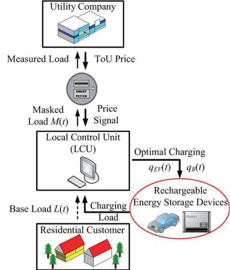
Fig. 1. An EV-assisted battery load hiding framework.
