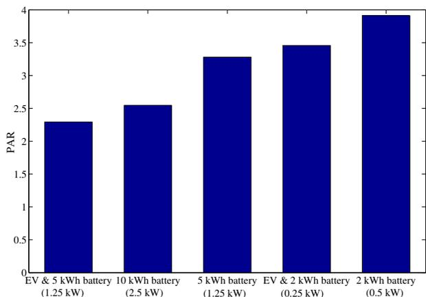
Fig. 7. Comparison of PAR for different batteries (maximum charging rate  $q_B^{\max}$ ) with and without the use of an EV for load hiding.
