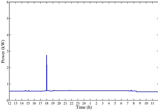
Fig. 4. The observed household load profile using a 5 kWh local rechargeable battery and an EV for load hiding.
