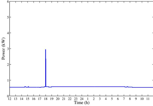
Fig. 3. The observed household load profile using a 10 kWh local rechargeable battery for load hiding.
