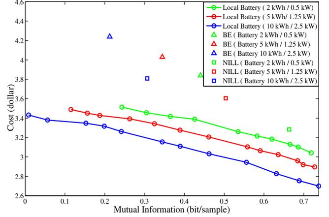
Fig. 5. Cost versus mutual information for different algorithms and batteries (maximum capacity  $C_B$  / maximum charging rate  $q_B^{\max}$ ).
