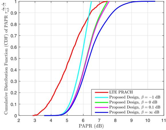
Fig. 5. The CDF of the PAPR for different values of tolerance threshold  $\beta$ . As  $\beta$  decreases, we select preamble pairs with lower PAPRs which enhances the PAPR performance but reduces the number of available preamble pairs.
