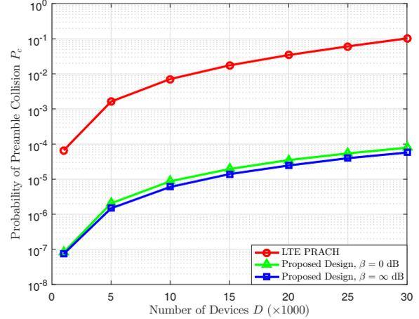
Fig. 6. The probability of preamble collision versus  $D$  for different preamble sequence designs with uniform arrival process and retransmissions.
