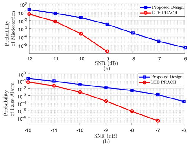
Fig. 8. (a) The probability of misdetection versus SNR. (b) The probability of false alarm versus SNR.
