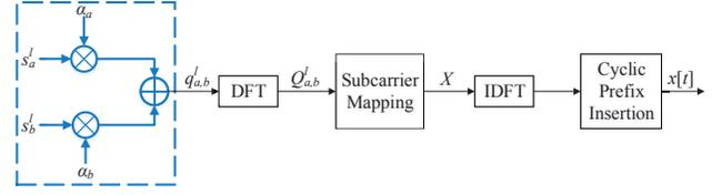
Fig. 2. Transmitter: Preambles  $s_a^l$  and  $s_b^l$  are scaled by  $\alpha_a$  and  $\alpha_b$ , respectively, and aggregated together. The resulting preamble sequence  $q_{a,b}^l$  is subject to DFT, subcarrier mapping, IDFT, and cyclic prefix insertion.
