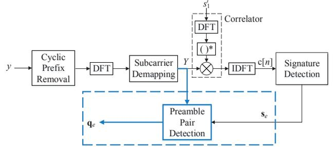
Fig. 3. Receiver: The received signal  $y$  is correlated with root sequence  $s_1^l$  to obtain time correlation  $c[n]$  that is used to estimate the transmitted preambles, i.e., set  $s_e$ . The preamble pair detection calculates the correlation between the received signal in the frequency domain and the subset of preamble pairs that can be generated using the preambles in set  $s_e$  to estimate the transmitted preamble pairs in set  $q_e$ .
