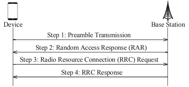
Fig. 1. Contention-based random access procedure in LTE-A systems [12].
