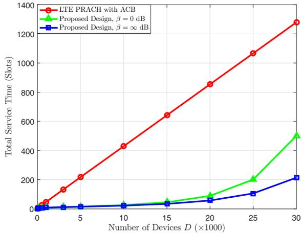
Fig. 7. The average total service time versus the number of devices  $D$  for different preamble sequence designs.
