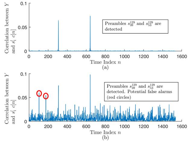
Fig. 4. Sample of correlation function  $c[n]$ . (a) In the absence of delay, noise, and channel fading, the transmitted preambles are detected successfully without any false alarms. (b) With AWGN and ETU fading channel, the receiver may detect false alarms (red circles).
