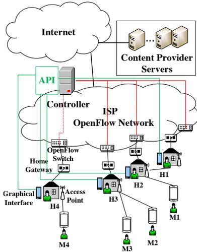
Fig. 1. Illustration of SDN-enabled network topology.
