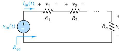
$$v_j(t) = \frac{R_j}{R_1 + R_2 + \dots + R_n} v_{in}(t)$$
