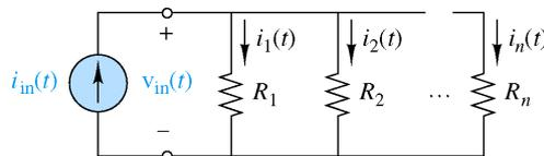
$$G_{eq} = G_1 + G_2 + \dots + G_n \quad \text{or} \quad \frac{1}{R_{eq}} = \frac{1}{R_1} + \frac{1}{R_2} + \dots + \frac{1}{R_n}$$
