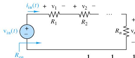
$$R_{eq} = R_1 + R_2 + \dots + R_n \quad \text{or} \quad \frac{1}{G_{eq}} = \frac{1}{G_1} + \frac{1}{G_2} + \dots + \frac{1}{G_n}$$
