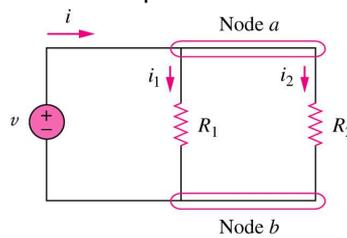
$$R_{eq} = \frac{R_1 R_2}{R_1 + R_2}, \quad i_1(t) = \frac{R_2}{R_1 + R_2} i(t), \quad \text{and} \quad i_2(t) = \frac{R_1}{R_1 + R_2} i(t)$$
