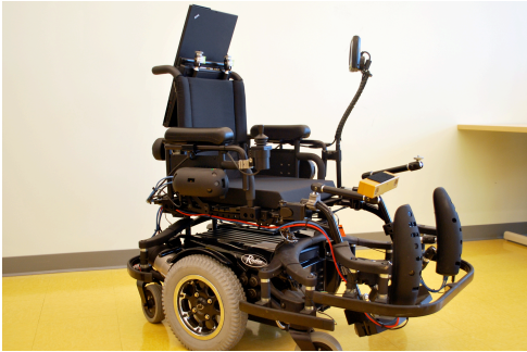
Figure 1: Quickie Rhythm with wheel encoders, bumper skirt, stereovision camera, and five sensor pods containing infrared and sonar rangefinders.
