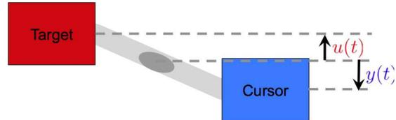
Figure 4: Experimental setup. The target trajectory is  $u(t) = \sin(\omega_1 t) + \sin(\omega_2 t)$ . Users are instructed to keep the cursor  $y(t)$  level with the target. The error  $u(t) - y(t)$  is scaled by 0.3 in ‘Better’ mode, by 2.0 in ‘Worse’ mode, and unchanged in ‘Normal’ mode.
