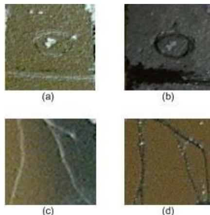
Fig. 3. (a,c) scratches on opposite sides of a p-type silicon wafer before electrodeposition. (b,d) electrodeposited polypyrrole inside the scribe marks. The diameter of circle in a and b is 2mm and the length of the lines in c and d is approximately 6mm.
