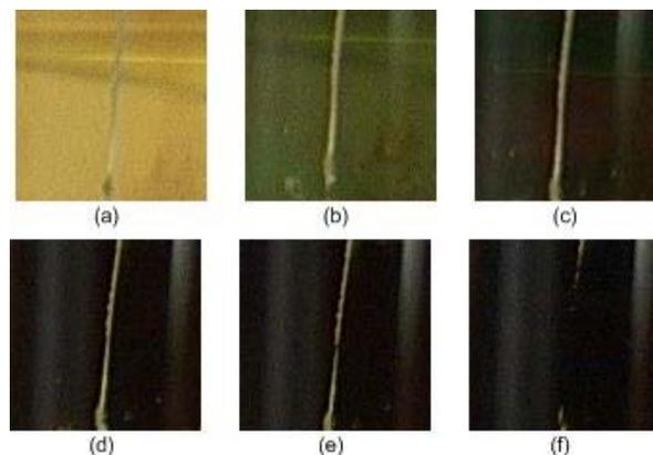
Fig. 1. Electrodeposition of polypyrrole on gold electrodes (gap=100 $\mu\text{m}$ ) with glass substrate at (a)0h (b)0.1h (c)1h (d)3h (e)5.5h (f)13h after the beginning of process
