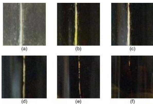
Fig. 2. Electrodeposition of polypyrrole on graphite electrodes (gap=1mm) with a paper substrate at (a)0h (b)1.5h (c)6h (d)9h (e)12h (f)15h after the beginning of process.
