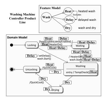
Figure 1: Example washing machine controller product line W.
