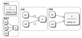
Figure 2: The "fold incoming actions" rule  $R_F$  for refactoring a state machine.
