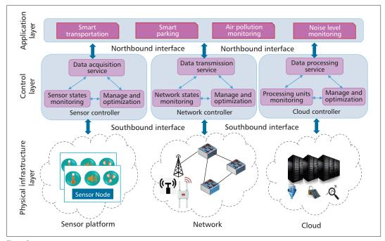
Figure 3. Architecture of software-defined IoT.
