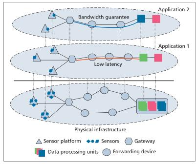
Figure 1. Illustration of software-defined IoT solution.
