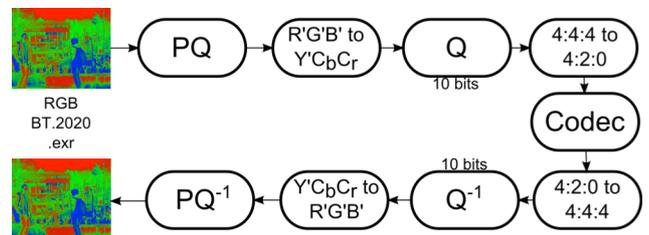
Fig. 1. MPEG workflow for encoding/decoding HDR streams
