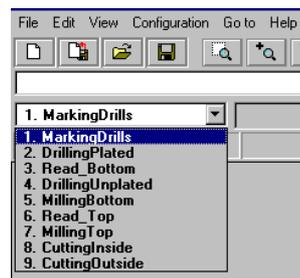
Select the production phase to be processed next. Ensure that only one production phase is marked to which an HP-GL file or LMD file has also been assigned. Erroneous selection leads either to erroneous files being processed or no data being transmitted at all.
