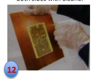
Remove oxide layer with brush
