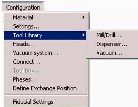
The tool library contains the definitions of all necessary tools inclusive their characteristic features for the circuit board plotter operation. To add tool or change existing tools the following parameter description must be observed.
