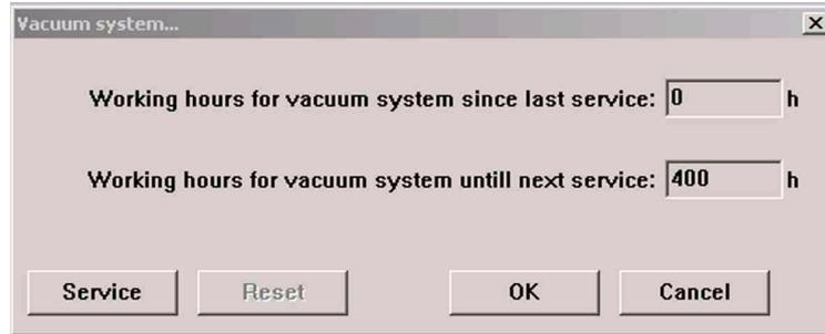
Use the submenu **VACUUM SYSTEM** to call up the status of the vacuum system. The operation hours will be reported.
