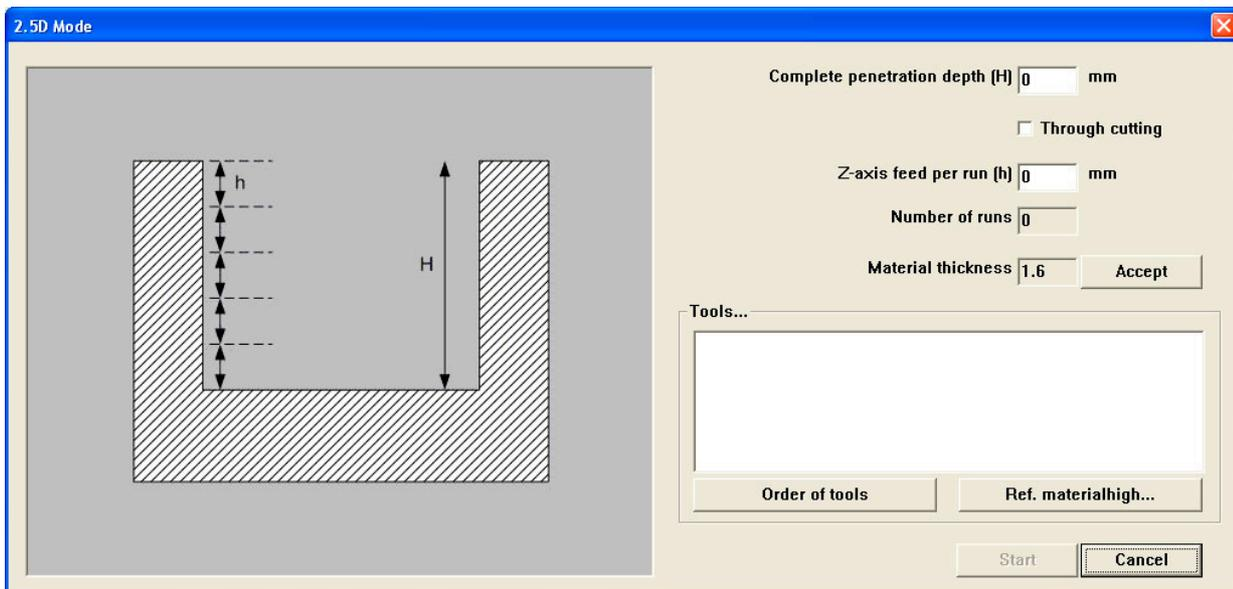
The material thickness is divided into various processing layers. The number of layers depends on the depth with which the tool penetrates the material. The penetration depth must be individually adapted to each tool. The settings that are made can be stored in the job.
