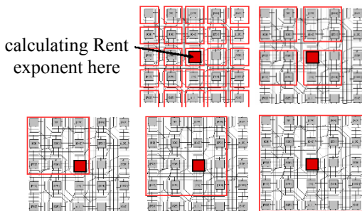
Figure 3: Calculating the Rent exponent for each CLB using a placement approach is demonstrated with a 5x5 window.
