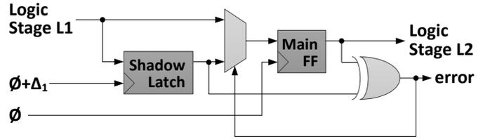
Figure 1. Razor shadow register and error detection
