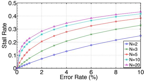
Figure 8. Fraction of performance stalled due to errors ( $N \times N$  array).
