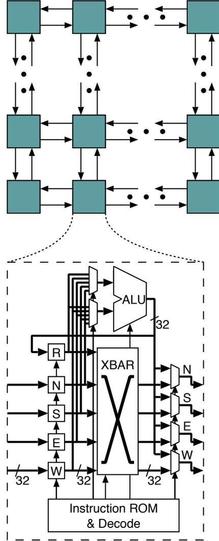
Figure 2. The tiled MALIBU architecture with PE detail.
