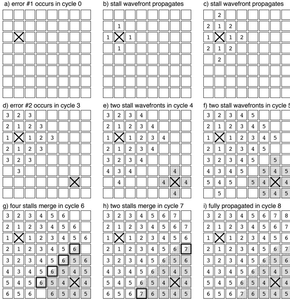
Figure 5. Error propagation in the 2D array, where two errors merge into a single stall cycle. Numbers indicate the clock cycle # of the stall.
