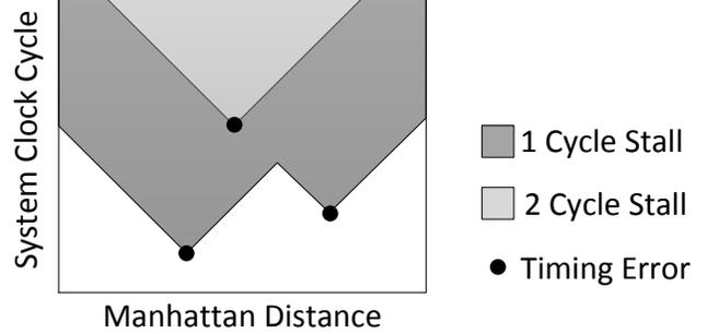
Figure 4. Conceptual graph demonstrating how 2 separate errors join to form one stall region, and how a later error creates a second stall.
