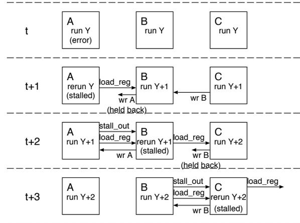
Figure 6. Proper stalling of writes into the wavefront.
