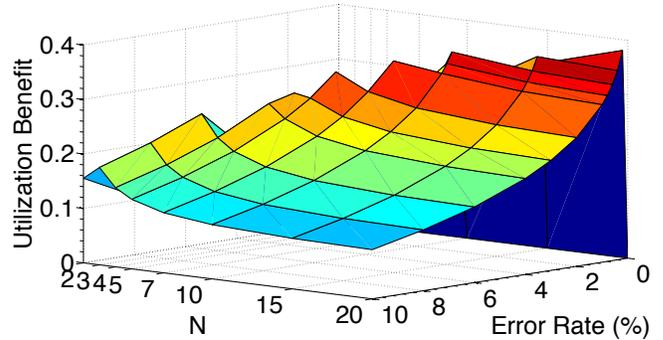
Figure 9. Gain in utilization due to merging of errors ( $N \times N$  array).
