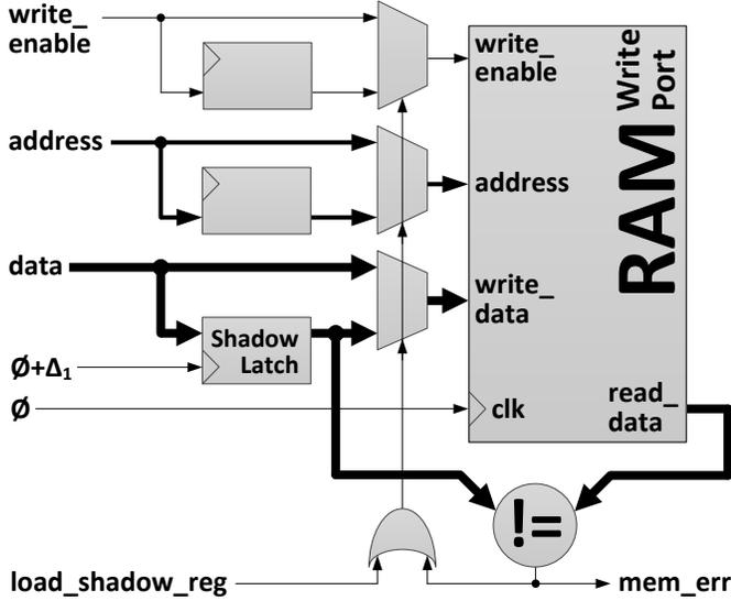
Figure 3. Shadow register applied to Stratix III memory
