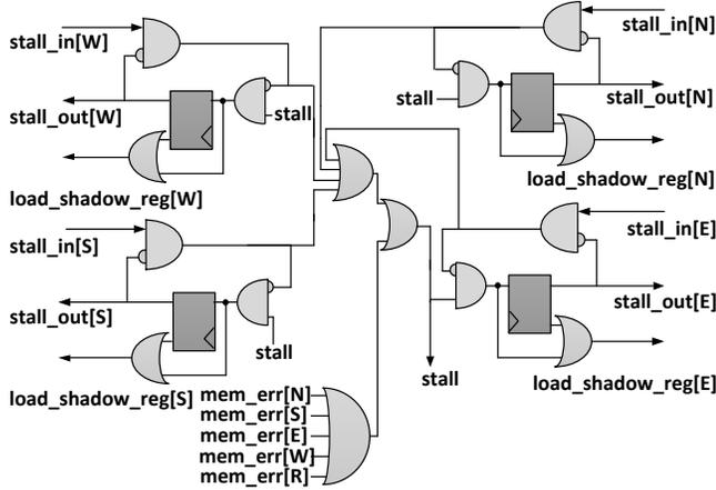
Figure 7. Control logic used to produce the stall signals in each PE.
