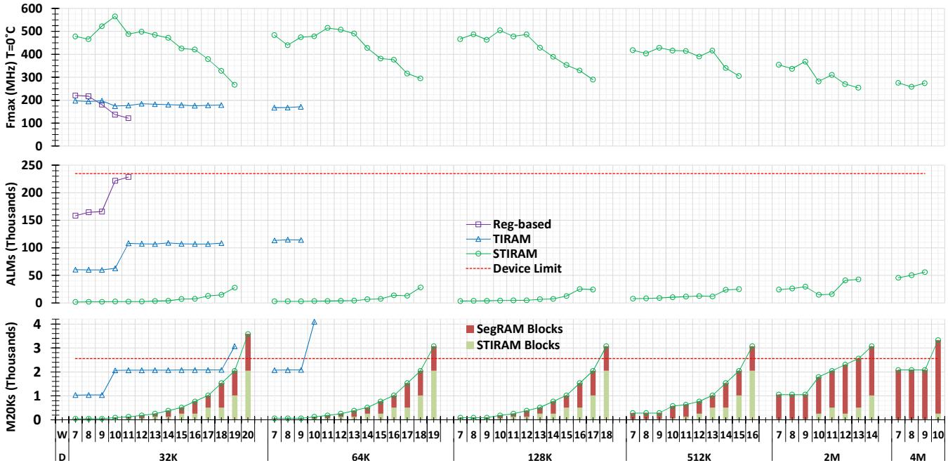
Fig. 4. Results for several BCAM depth and pattern width sweeps (bottom) M20K count (1000's) (middle) ALMs count (1000's) (top) Fmax (MHz) T=0°C
