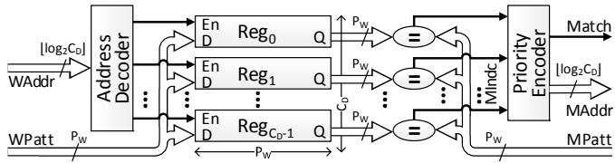
Fig. 1. Register-based BCAM
