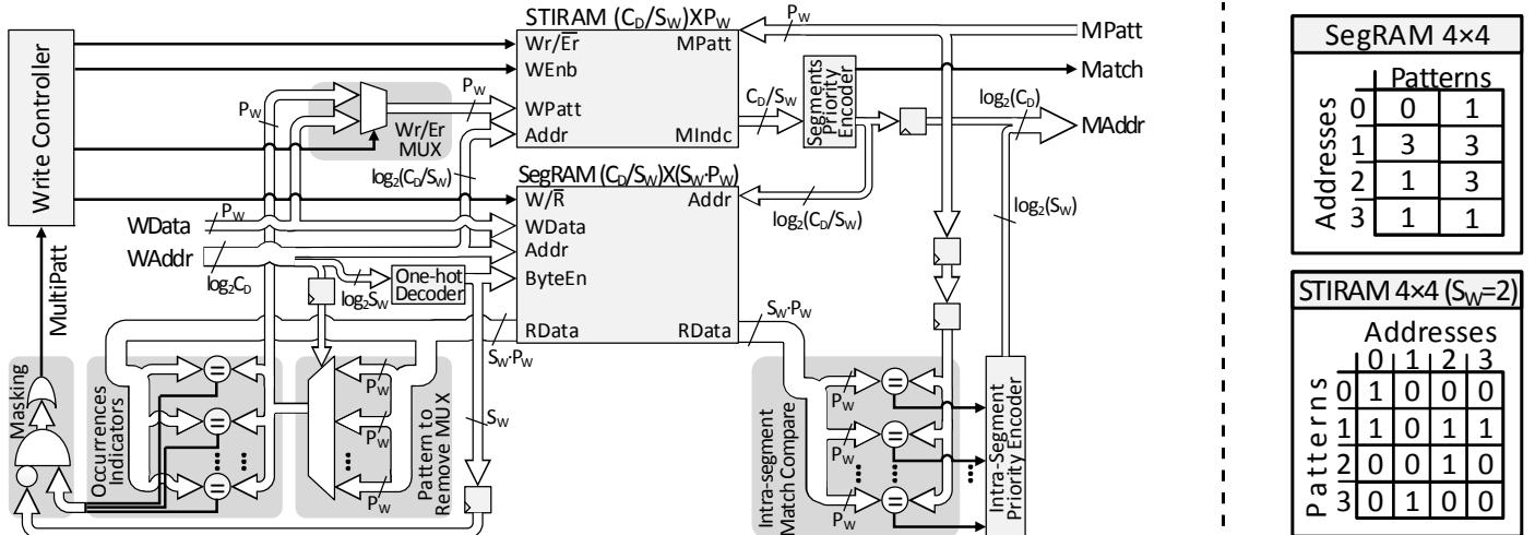
Fig. 3. (left) The complete STIRAM BCAM (right) 8×2;  $S_W=2$  example
