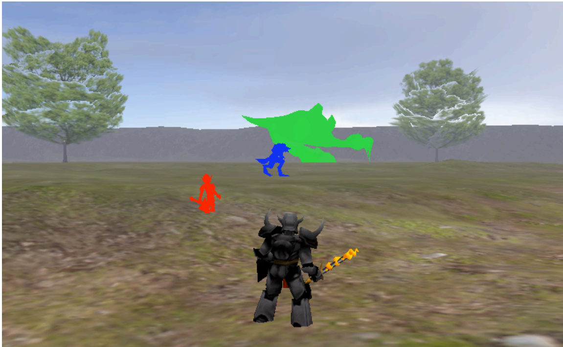
Figure 15: Example of monsters coloured with their unique colour used for colour picking.
