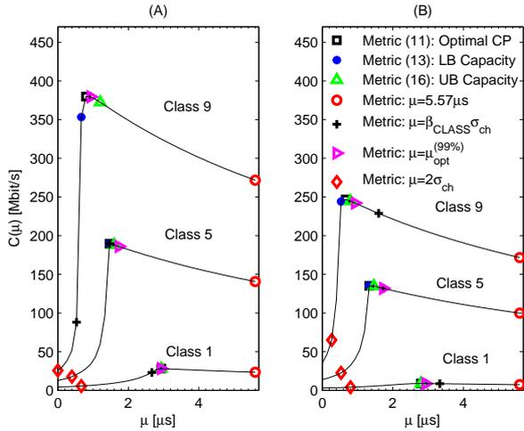
Fig. 3. Capacity  $C(\mu)$  as function of the CP length  $\mu$ , for different PLC channels. Markers indicate the CP length obtained from the different criteria proposed in Section III. Subplots (A) and (B) show the results for the best case and the worst case channel impulse responses, respectively.
