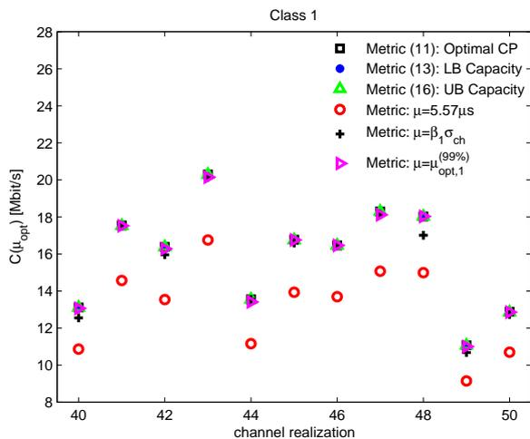
Fig. 5. Capacity  $C(\mu)$  for  $\mu$  optimized according to the different criteria presented in Section III as function of the channel realization belonging to Class 1. For the sake of readability, only realizations 40 to 50 are shown out of 100 realizations.
