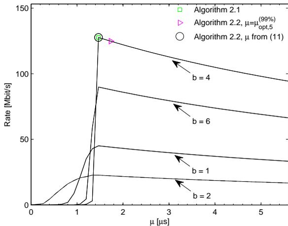
Fig. 9. Bit rate  $R(\mu, b)$  from (24) as function of CP length  $\mu$  and constellation size  $2^b$  for uniform bit-loading. Markers are results from Algorithms 2.1 and 2.2 from Section IV-B. The BeC channel of Class 5 is assumed. The system uses 384 sub-channels.
