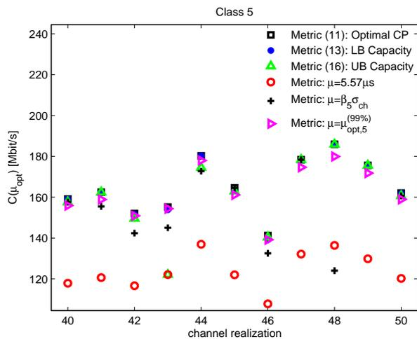
Fig. 6. Capacity  $C(\mu)$  for  $\mu$  optimized according to the different criteria presented in Section III as function of the channel realization belonging to Class 5. For the sake of readability, only realizations 40 to 50 are shown out of 100 realizations.
