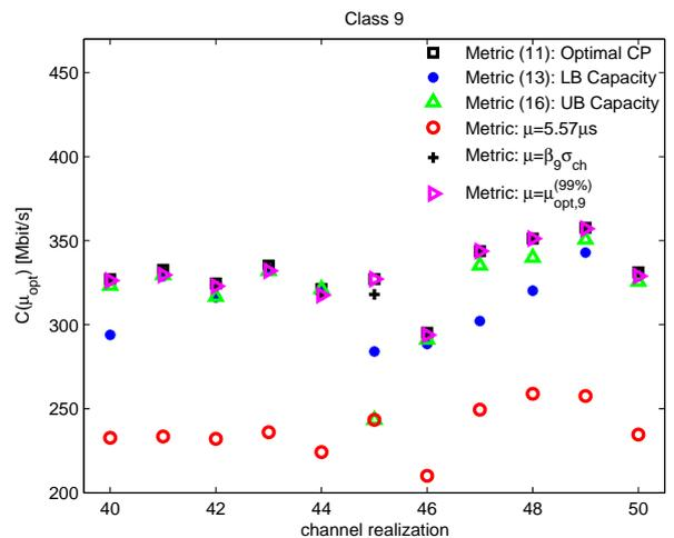
Fig. 7. Capacity  $C(\mu)$  for  $\mu$  optimized according to the different criteria presented in Section III as function of the channel realization belonging to Class 9. For the sake of readability, only realizations 40 to 50 are shown out of 100 realizations.
