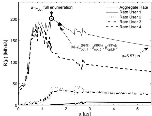
Fig. 10. Aggregate and single user rate using bit-loading as a function of the CP length. The OFDMA system has  $N_U = 4$  users and  $M = 384$  sub-channels. The users experience channels belonging to different classes. Markers are results from Algorithm 3 from Section V with different sets of CP length  $\mathcal{M}$ .
