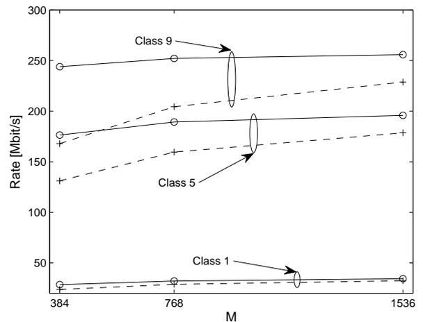
Fig. 8. Capacity  $C(\mu)$  for bit loading with Algorithm 1.2 of Section IV-A and  $\mu$  optimized according to the capacity-optimal criterion (11) and three different numbers of OFDM sub-channels  $M \in \{384, 768, 1536\}$ . For a comparison,  $C(\mu)$  for bit loading and  $\mu = 209$  (corresponding to  $5.57 \mu s$ ) is also included. The channels employed are the BeC channels of the three used classes.
