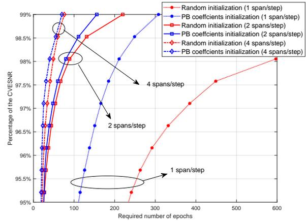
Fig. 3: PA-LDBP convergence behaviour with different initializations.
