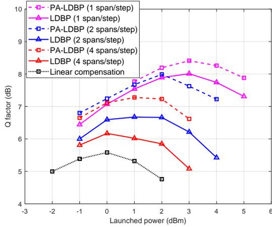
Fig. 2: Performance of PA-LDBP (dashed line) and LDBP (solid line).
