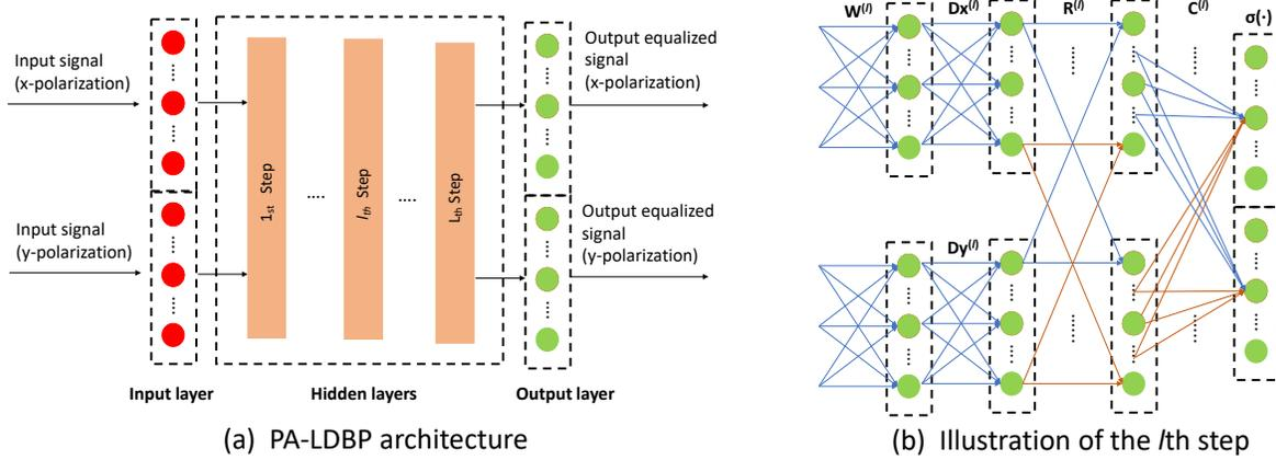
Fig. 1: Diagram of the proposed PA-LDBP.
