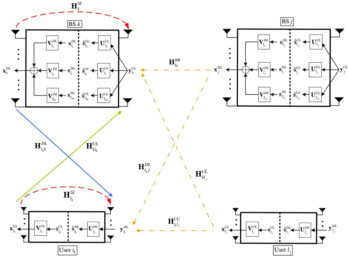
Fig. 1. Full-duplex MIMO multi-cell system. Dashed arrows denote the self-interference and the dash-dotted arrows denote the interference between different nodes.
