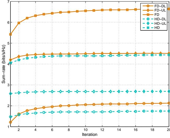
Fig. 6. Convergence of minimum SINR i.e., improved associated rate in the presence of imperfect CSI with  $s = 0.02$  and  $\kappa = \beta = -120\text{dB}$ .
