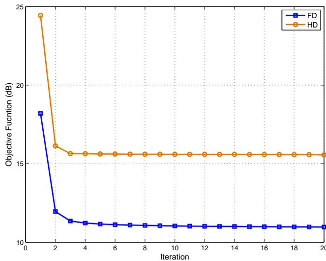
Fig. 2. Convergence of the objective function in (29) for perfect CSI design with  $\kappa = \beta = -120$ dB.
