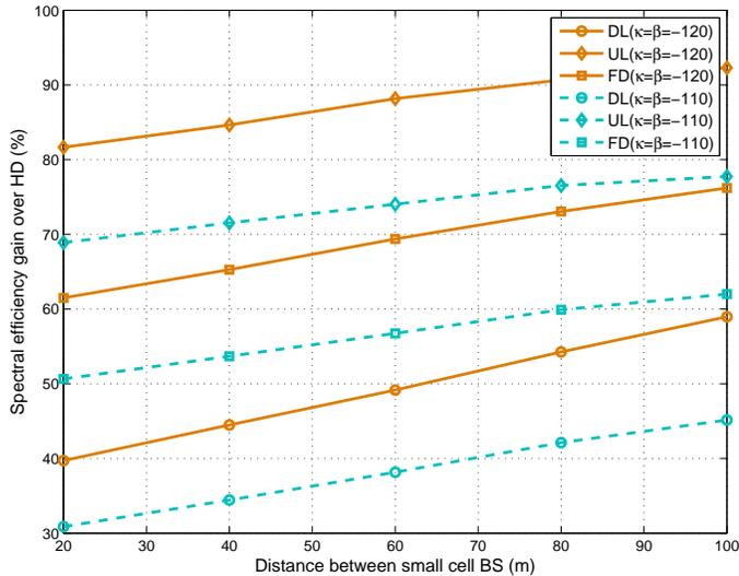
Fig. 4. Total sum-rates achieved for FD and HD setups with perfect CSI and varying distance between BSs. The parameters representing transceiver distortion are chosen as  $\kappa = \beta = -110\text{dB}$  and  $\kappa = \beta = -120\text{dB}$
